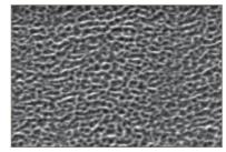
Parker's Global Shield coating features a sub-micron structure (shown here magnified 4000 times) that eliminates surface micro-cracks and delamination.
